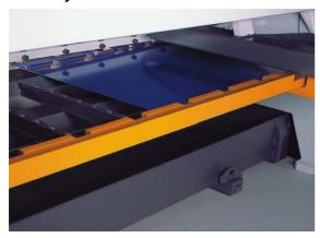
This shear is designed especially for application requiring flexibility and cutting of small batch sizes. An unique integrated sheet support, sort and stacking system provides optimum management of cut pieces. This system automatically separates scrap from cut pieces and can sort the desired pieces in four different stacks. The system can also return a cut piece from the rear back to the operator. This eliminates the operator walking to the rear to retrieve a cut piece for the next operation.
