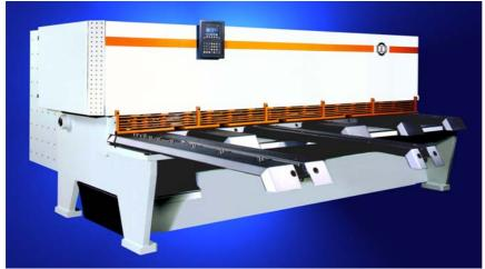
The hydraulic swing beam shear RAS POWERcut cuts sheet metal thicknesses up to 6.3mm. The CNC control positions the automatic backgauge at high speeds to an accuracy of +/- 0.1mm.
