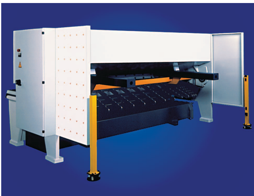
Sorting and sheet support system at the rear of the machine.
