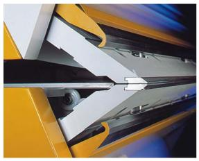
That's it. The machine automatically inserts, squares, positions to the bend line, and bends the flanges up or down. No more rotation. No more complicated handling. No more second or third operator. You've got automatically produced precision parts, in record time! And, be-
