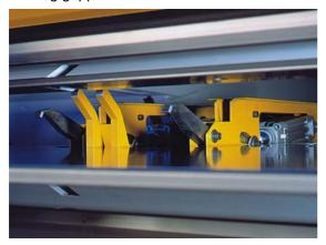
The feeding grippers hold the part during the entire bend cycle and position it automatically for each bend. For most parts the operator unloads only the finished workpiece. Only on parts with hems on both sides does the operator flip the workpiece once during the bend cycle. Even then, rotating the part is not required.
