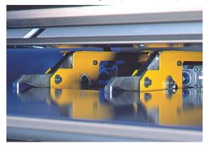
Hems should be closed to a programmable dimension. The operation of the machine should be as simple as possible, so that even less experienced operators can use the machine. The feeding grippers can clamp on straight material, but can also clamp above a pre-bent hem or a closed hem. Each gripper unit sits on a separate guiding system with high precision linear guides. This guarantees precision and accurate flange dimensions and a high speed, dynamic drive characteristic.
