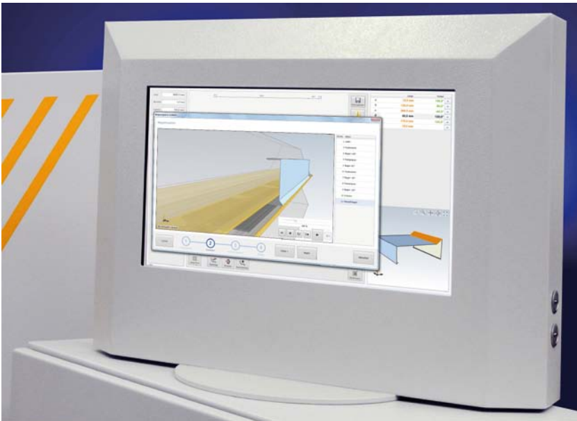
The PC control simulates the folding sequence in 3D
