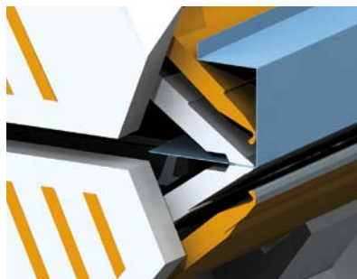
The form fitting folding beams create large free spaces and allow the beams to dive into pre-bent profiles.
