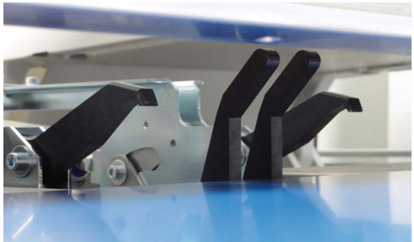
Pneumatically operated pop-up stop fingers automatically square the blank.
