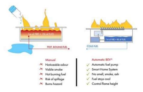
Automatic BEV® technology guarantees complete separation of the fuel tank and fire. This, coupled with multiple sensors, meets even the most robust safety requirements.
