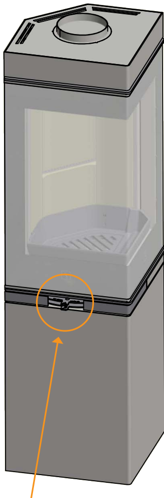
Dampers for primary- and secondary air
